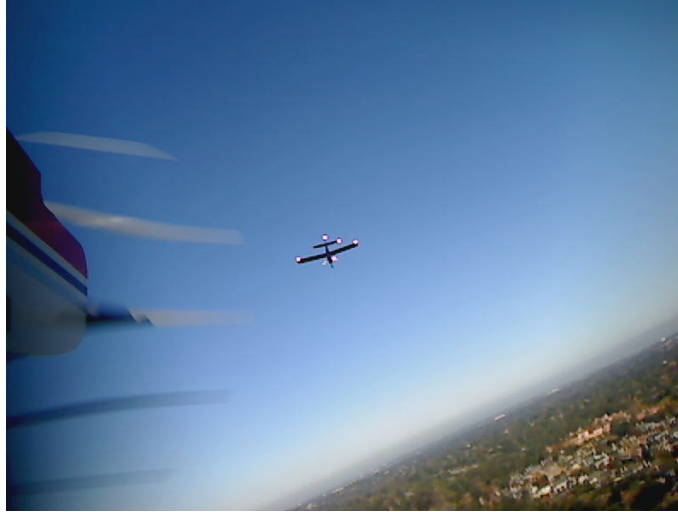
Figure 10. View from the camera on the trailing aircraft. The red dots on the lead aircraft are high power LEDs used for relative positioning.
