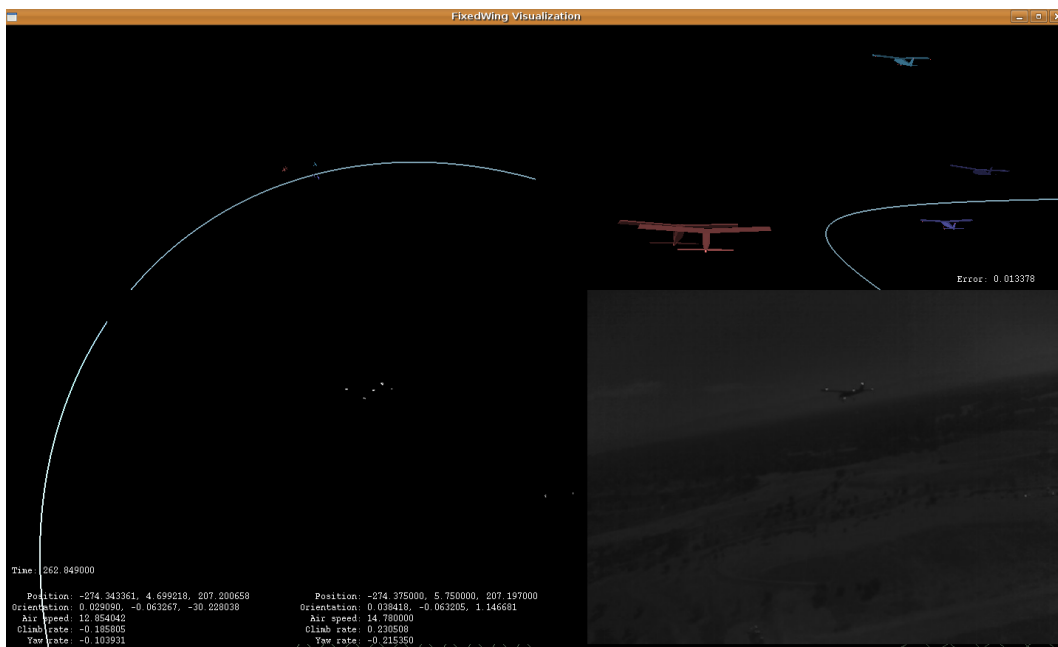
Figure 13. Screenshot of the custom GUI with camera view in the bottom right, filtered image in the bottom left and position estimates in the top (camera view only available in flight log-replay mode)
