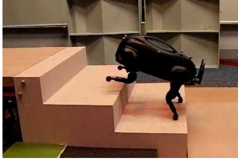
Figure 15: The desired task for the LittleDog: climb over three large steps.
