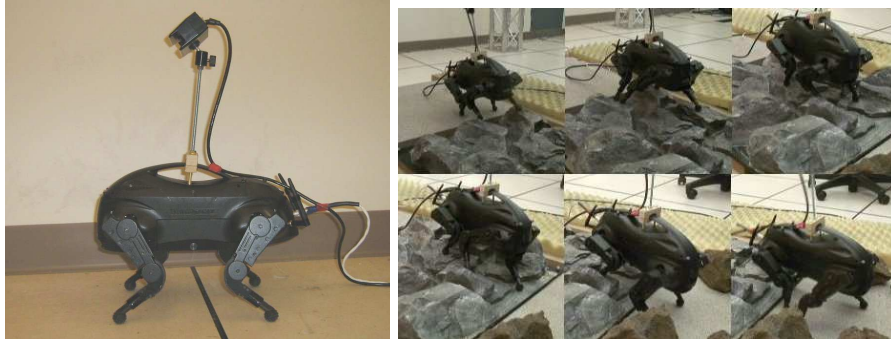
Figure 17: Prototype system with onboard stereo camera, and snapshots of the system crossing one of the more difficult terrains, using only onboard vision.
