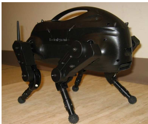
Figure 1: The LittleDog robot, designed and built by Boston Dynamics, Inc.
