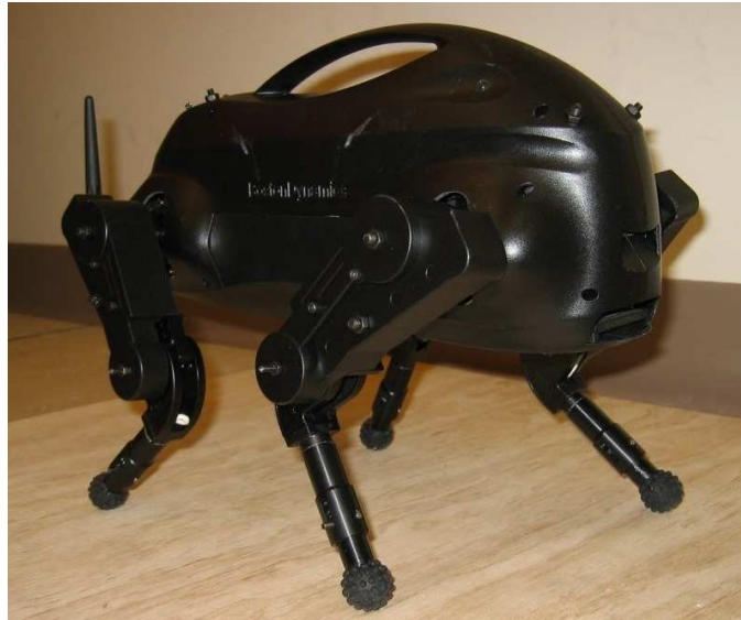
Figure 6.1: The LittleDog robot, designed and built by Boston Dynamics, Inc.
