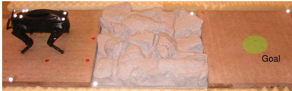
Figure 6.2: Typical quadruped locomotion task: navigate robot over terrain to goal.
