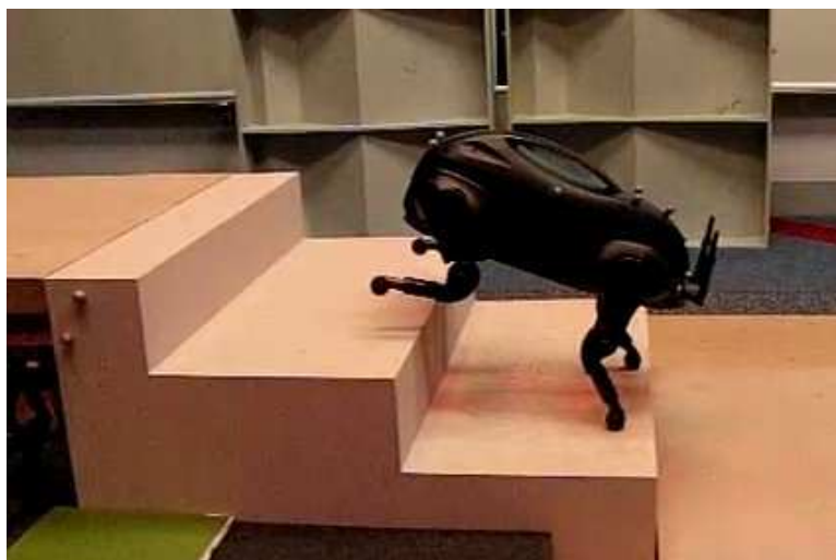
Figure 3.10: The desired task for the LittleDog: climb over three large steps.
